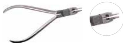
Kim plier Item No.: FC06-01 Package: 1*1 For bending multi-loop edgewise arch wires. With cutter in the middle part. For rectangular wires not up to 0.022". three step loop formers are 1.5mm, 2mm, 2.6mm.
